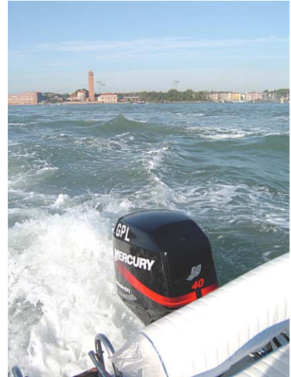
▲ Pic. 1 – The first boat of the demonstration fleet fitted with an LPG/petrol bifuel engine circulating in the Venice lagoon
