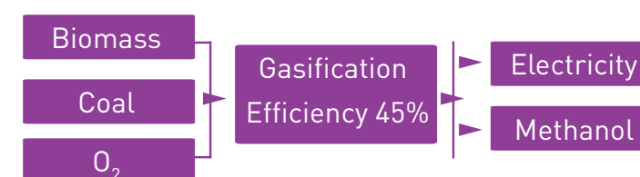
Simplified diagram of biomass gasification methanol synthesis system
